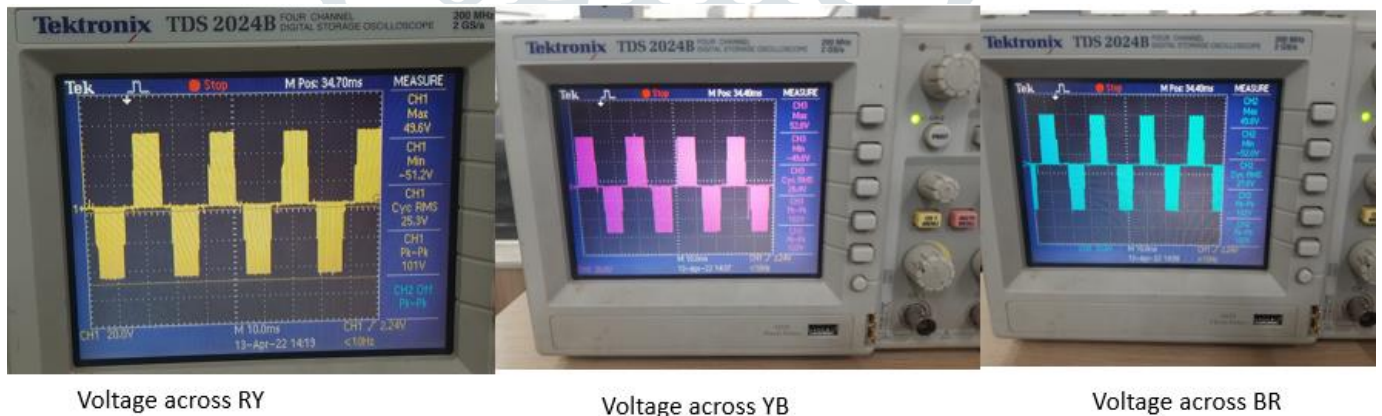
Fig.20 Line Voltages across RY, YB and BR terminals of the DUT motor on no-load
