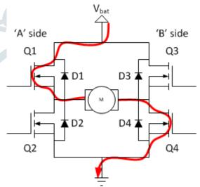
Bi-polar or FET transistors, or IGBTs in some high-voltage applications, typically serve as the switching elements (Q1– Q4). The catch diodes (D1..D4) are typically Schottky-type semiconductor devices. The bridge's bottom end is grounded, while the top end is wired to a power source (a battery, for instance). Although there are certain obvious limitations, generally speaking, all four switching parts can be separately turned on and off.
