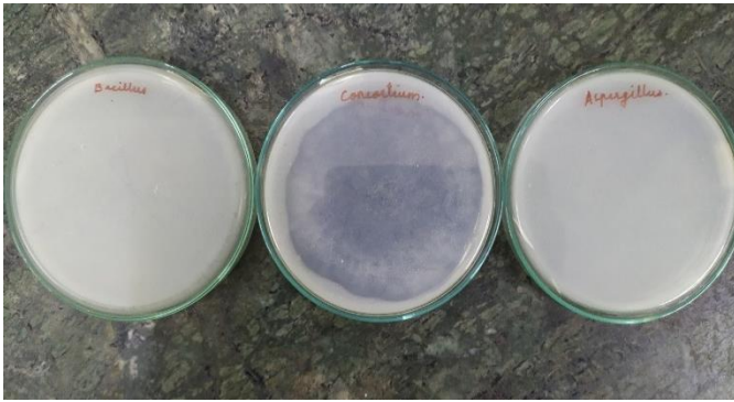
Fig 3: Clear zones produced by the consortium of Aspergillus and Bacillus in Carbonate Dissolution test.
