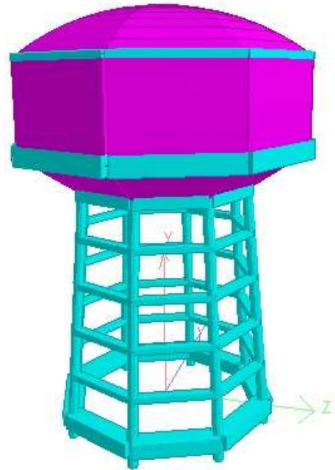
Figure 5.2: Intze tank 3D model
