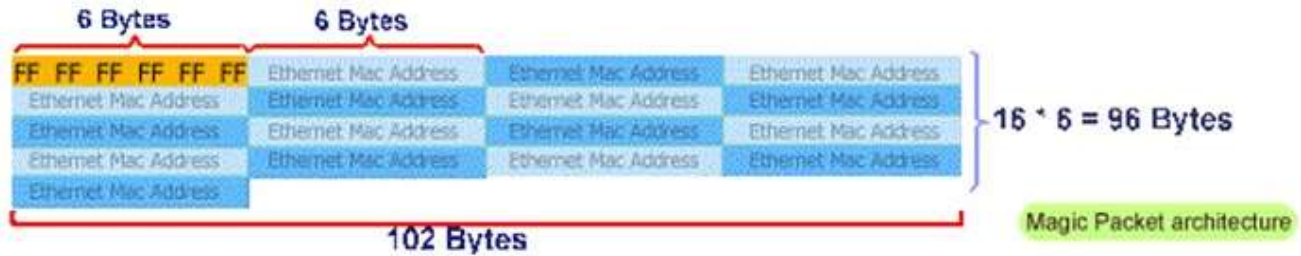
Figure 2: Magic Packet Architecture
