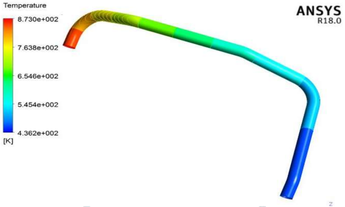
Figure 3. Analysis of pipe 1 original
