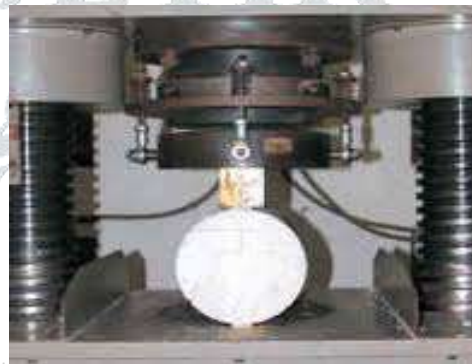
Fig 5 Testing of cylinder
