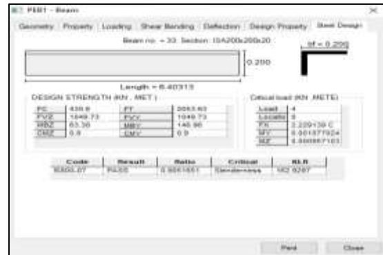
Figure 10: Checking beam for safety
