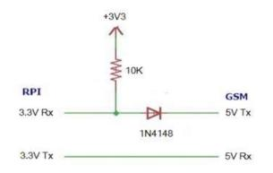
Fig 2: Level Shifter Circuit
