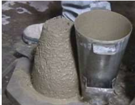
Fig: Slump cone test.
