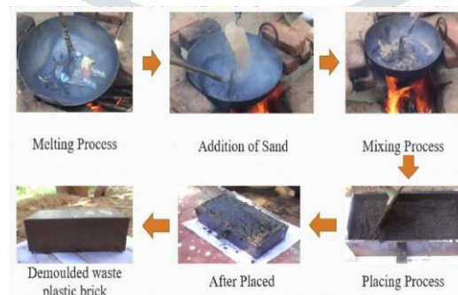
Fig 2: Preparation Process of Plastic Soil Brick
