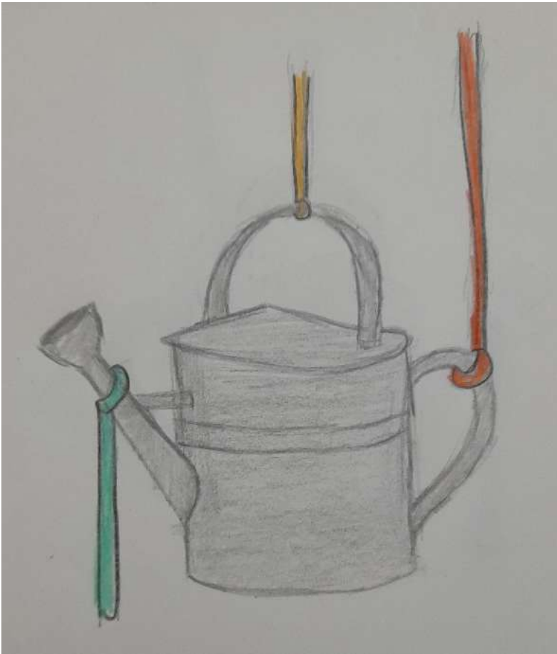
Figure 4: String C used to secure the handle of the dispenser
