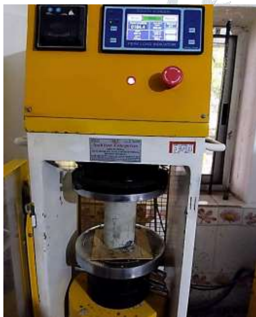
Fig 4: Semi-automatic Compressive testing machine
