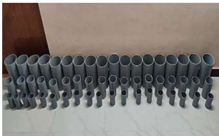
Fig 2: The PVC pipe molds with different sizes used for concrete samples.
