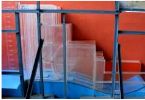
Figure 2: Model the of spillway
