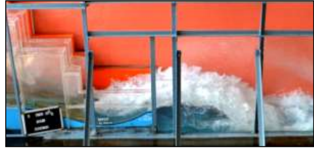
Figure 3: Flow conditions over the spillway for a discharge of 8750\text{m}^3/\text{s} , un gated operation of spillway
