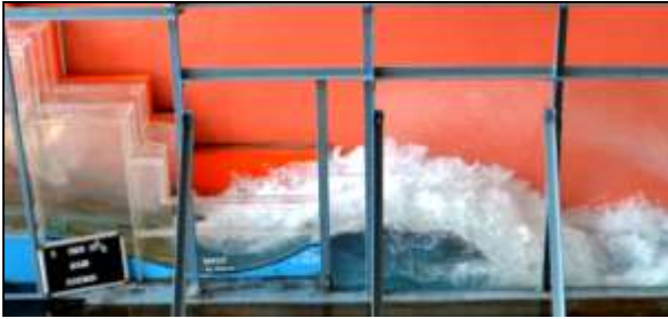
Figure 12: Photo showing flow conditions over spillway and energy dissipator for a discharge of 8750 m 3 /s for ungated operation of spillway
