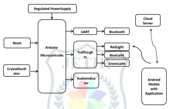
There are two modules in the system. Android applications make up the first module, which is a software module. The hardware module for traffic signal implementation is the second module.
