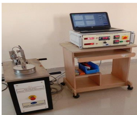
Fig.2 Experimental setup of Pin-On-Disc (Principle)
