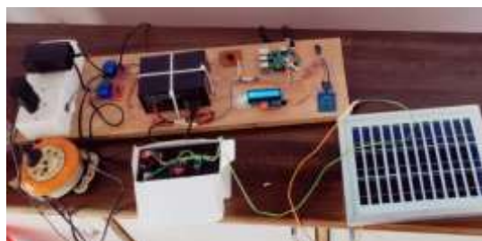
Fig 1: Model of EV charging station
