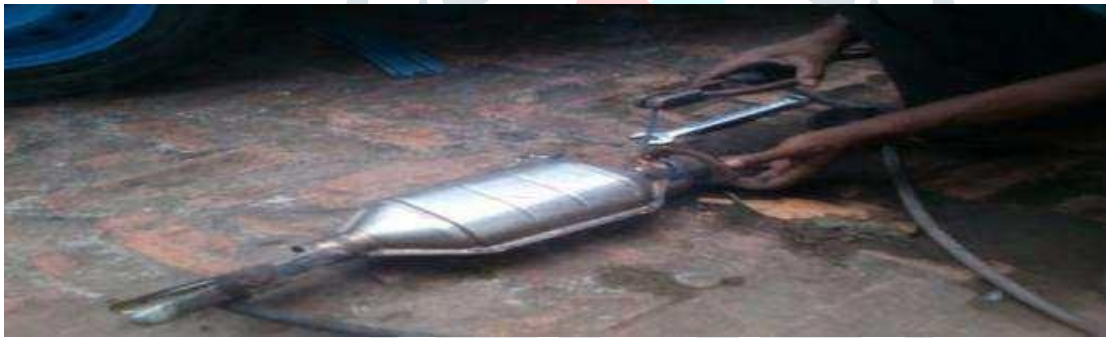
Fig 2: Catalytic converter to be welded in exhaust system of the car, Toyota E-90 in MIST welding shop.
