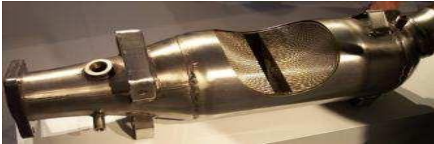
Fig 6.1: (a) Cutaway of a metal-core converter
