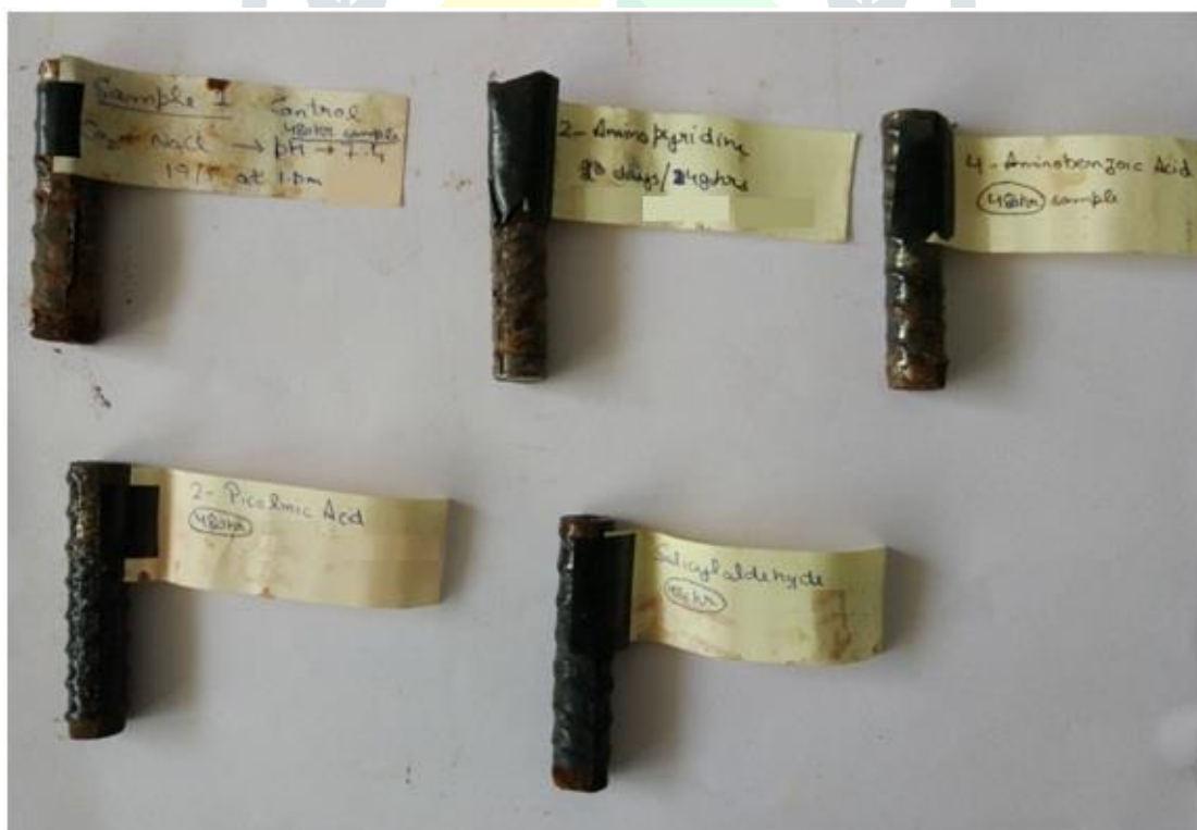
Figure 5.10: After 480 hours of immersion in various solutions, steel specimens were measured for half-cell potential and linear polarisation resistance.
