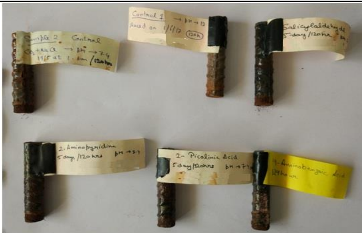
Figure 5.6: Steel specimens after measuring Half-cell Potential and Linear Polarization Resistance, immersed in different solutions after 120 hours
