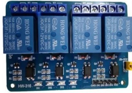
Fig.6 4 channel 12V relay module
