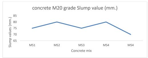
Fig.1. Slump value of concrete mixes of M20 grade
