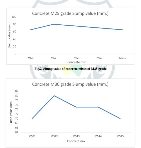
Fig.3. Slump value of concrete mixes of grade M30
