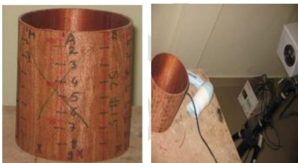
Fig 11: High Silica Phenolic Through Transmission experimental set up
