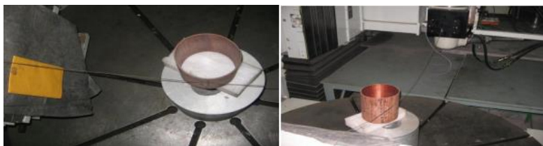
Fig 7: Tangential Radiography experimental set up
