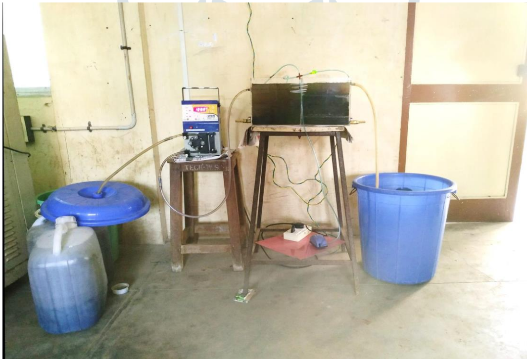
Figure. 1. Photographic view of Hybrid Aerobic Bio-Reactor
