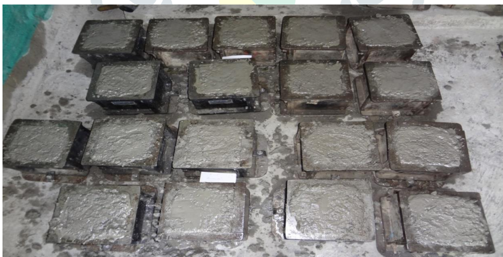
Fig: 1.1 Concrete Casted in Molds
