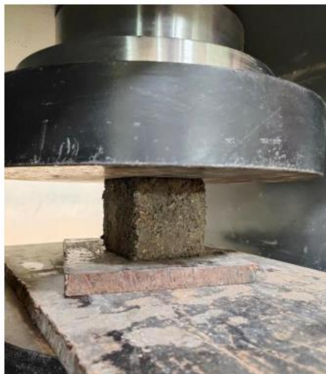
Fig 3. Compression test on Plastic Paver Block
