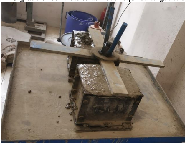
Figure 10: Prepared cube for compressive strength test.
