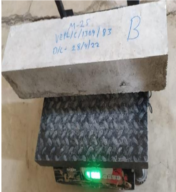
Figure13: Prepared beam for Flexural strength test.
