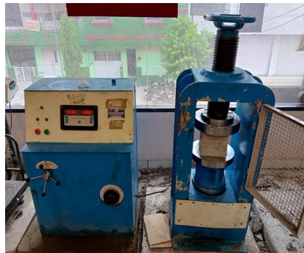
Figure 11: Load applied by Compression Testing Machine.
