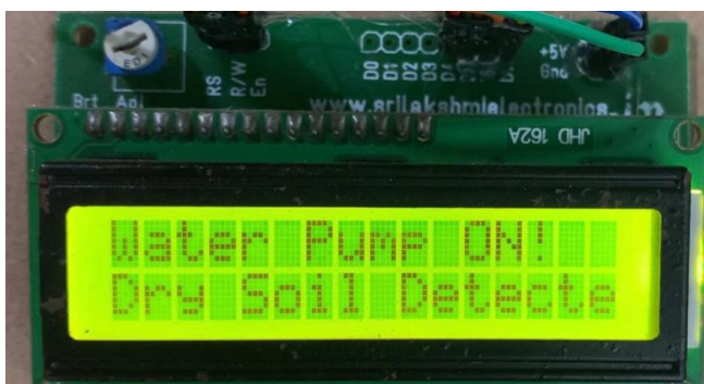
Fig.17: LCD shows that Water pump ON When Soil Dry
