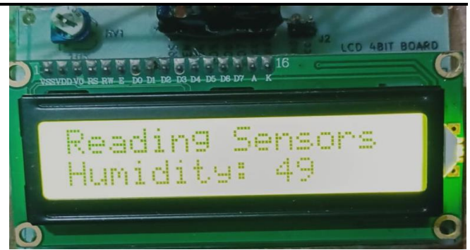
Fig.14: LCD shows that Humidity value
