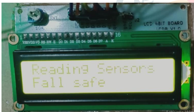
Fig.12: LCD shows that fall status detected when Gyro sensor activated
