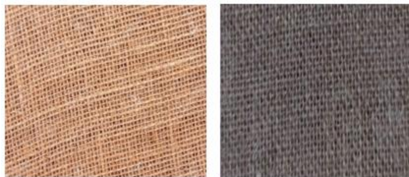
Fig 1: a) Jute fiber before treatment b) Jute fiber after surface modification
