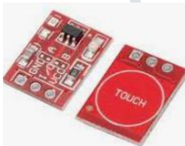
Fig.10: Touch sensor used as a switch
