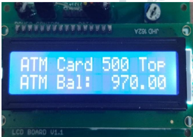
Fig.14: LCD Shows that ATM Card Balance When top up with ATM Card
