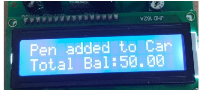
Fig.16: LCD Shows that When Pen added to cart and reduce the amount 50 Rs. from balance
