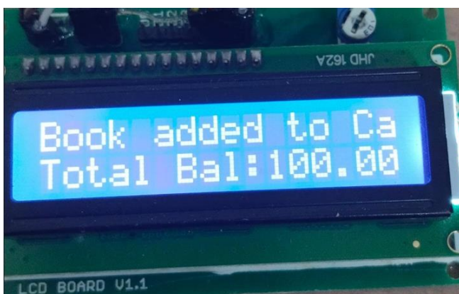
Fig.15: LCD Shows that When Book added to cart and reduce the amount 100 Rs. from balance
