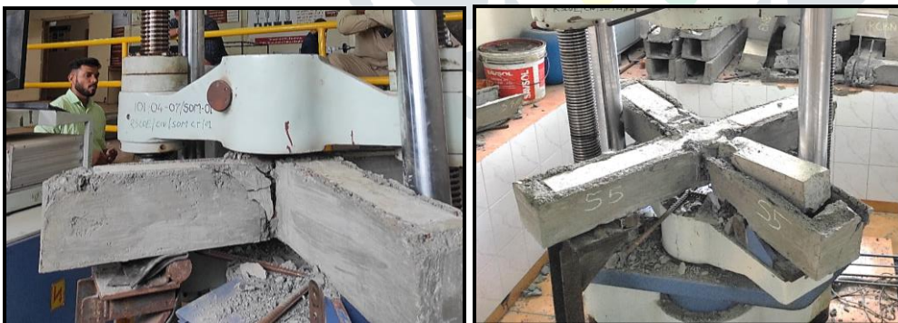
Fig. Ultimate Load Failure of Confined Ferrocement Cross-Beam
