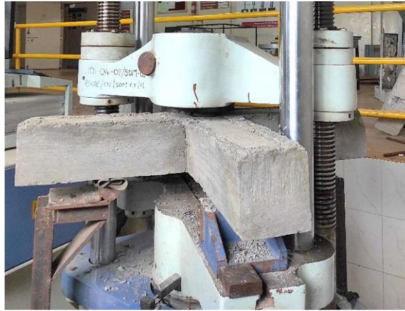
Fig. Placing of Cross Beam Specimens over Support System
