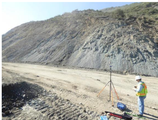
(fig. 2) GPS measurements in a landslide area
