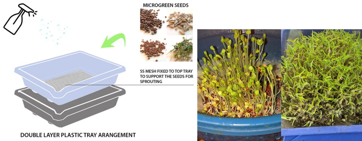
Figure 5: Illustration and Experimental results of the Tray systems
