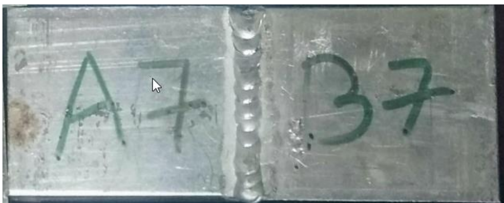
Fig 2. TIG welded joint of AA1100 and AA3003
