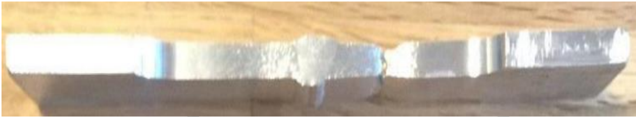
Fig 6. The picture shows fractured tensile samples on the cross-section side
