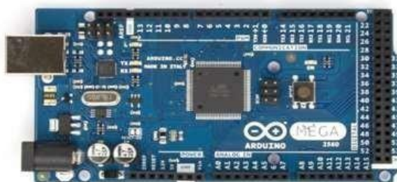
Fig.5 arduino mega (AT mega 2560) microcontroller unit
