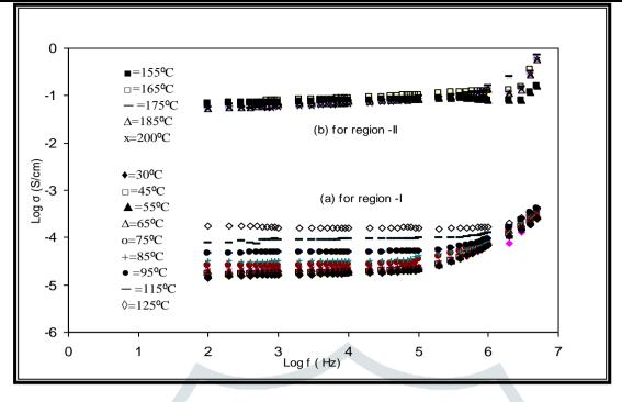
Figure 3 Log  $\sigma$  vs. log f plots for OCC: 0.85 [0.75 AgI: 0.25 AgCl]: 0.15 CeO2 (annealed) at different temperature
