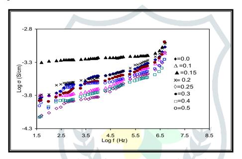
Figure 1. Log σ vs. log f plots for composite electrolyte system: (1-x) [0.75 AgI: 0.25AgCI]: x CeO2 at room temperature
