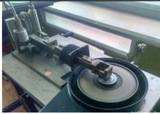
Figure 3.1: Pin on Disc Apparatus
