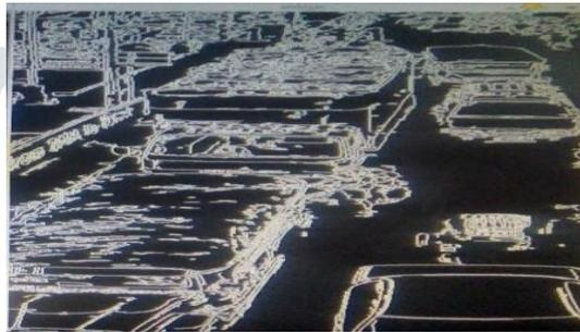
Fig. 5. picture that has been binarized and has edges identified
