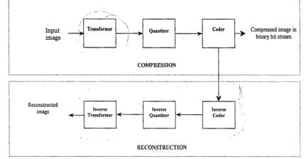
Figure 1: Elements of data compression and reconstruction model
