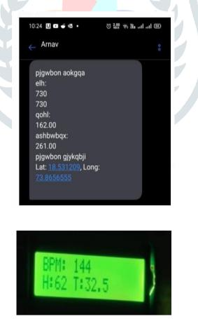
The LCD shows the actual values of the Soldier, i.e., his/her Pulse rate, temperature and humidity. But the SMS received by the information would have ciphered values and not the original one. These values are reverse engineered with the same key used for the encryption.
