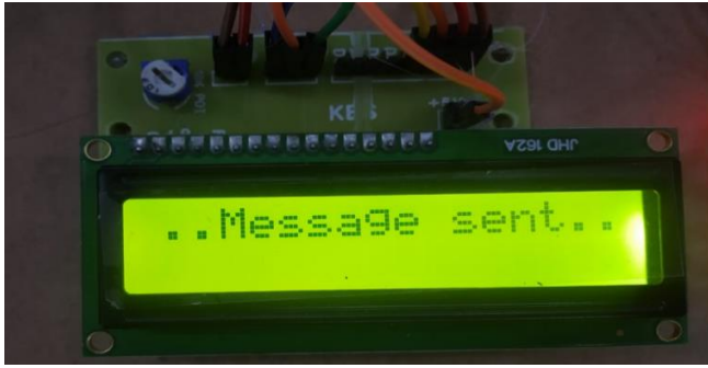
Fig.14: LCD Shows that message sent to concern department when fire detected
