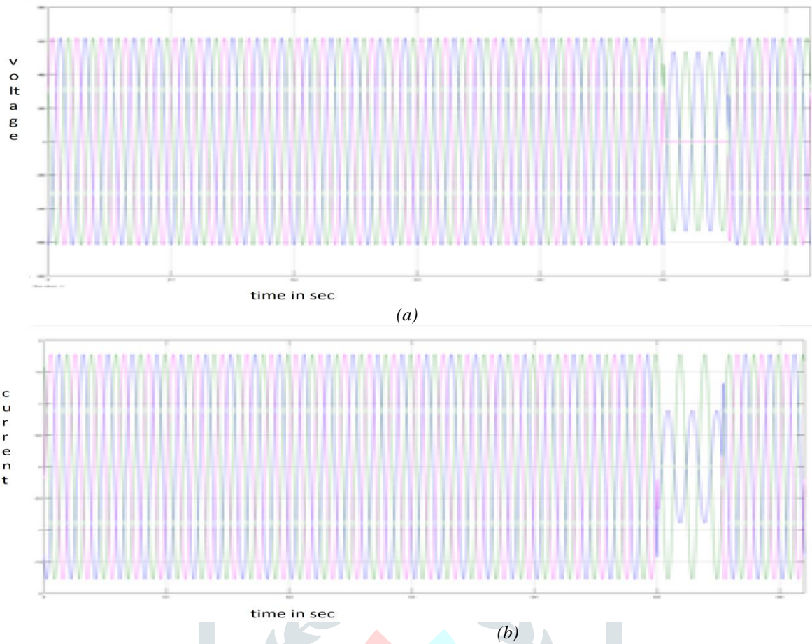
Fig.15. LG fault analysis (a) voltages (b) Currents. Here in fig.15. The line to ground fault occurred.
