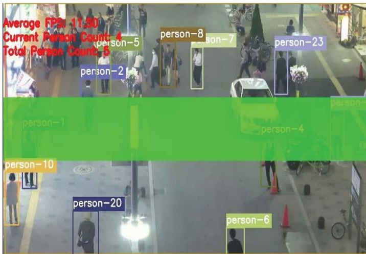
Fig. 4. The zone becomes green when the number of objects is less than 5.
