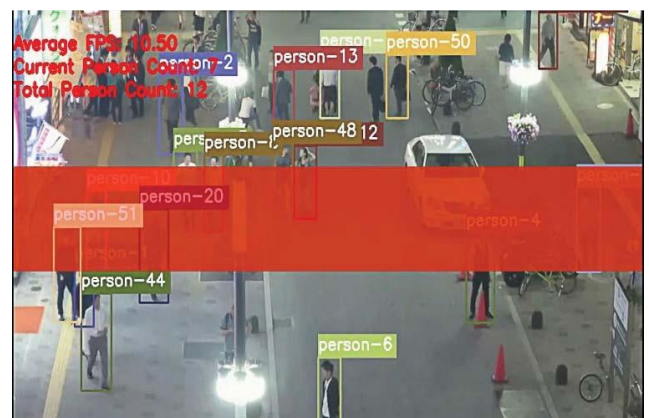
Fig.3. The zone becomes red when the number of objects is greater than or equal to 5.
