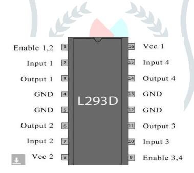
The L293D is a 16 pin IC, with eight pins, on each side, dedicated to the controlling of a motor. There are 2 INPUT pins, 2 OUTPUT pins and 1 ENABLE pin for each motor. L293D consist of two H-bridge. H-bridge is the simplest circuit for controlling a low current rated motor.
