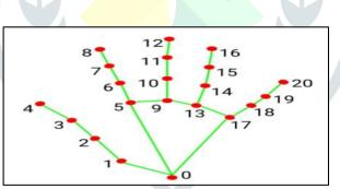
Fig 3. Hand Landmarks calculated using Mediapipe
