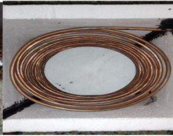
Copper Coil tube placed in refrigerator cabinet
