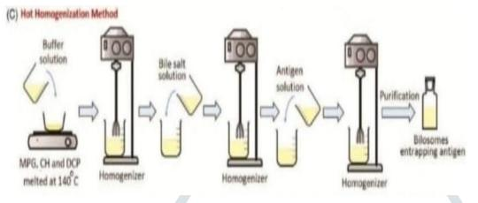
Figure 3: Hot homogenization method [38]
