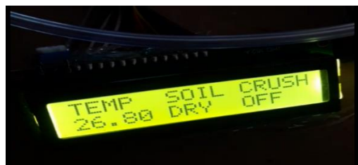
Figure:5 Indicates Temperature value & Soil status of compost
