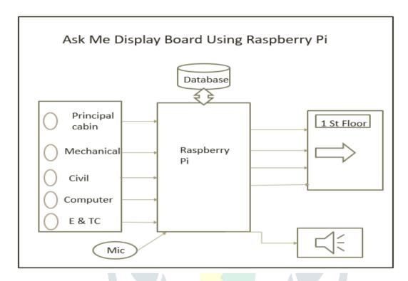
In this project, the Raspberry Pi is the main control unit, used to responsible for receiving user input through the keypad or button and displaying the corresponding information on the LED matrix display board. The Raspberry Pi interacts with the LED matrix through its GPIO connector's pins on the board. The keypad or button provides user input, which is read by the Raspberry Pi to determine what to display on the LED matrix.
