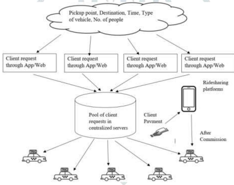
Fig. 1 Existing System of P2P Carpooling
